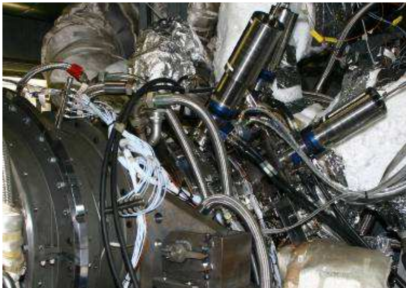
Rig on test stand with injection hoses and probes
