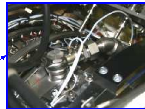
Close-up of air injection port
