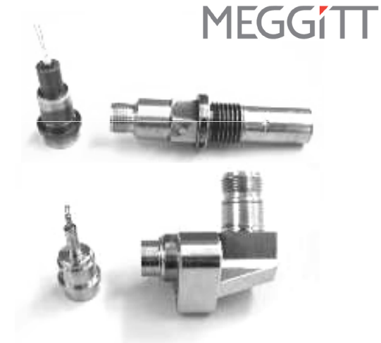
Two different prototype versions of fast pressure transducer to be used in NEWAC HPC rig test
