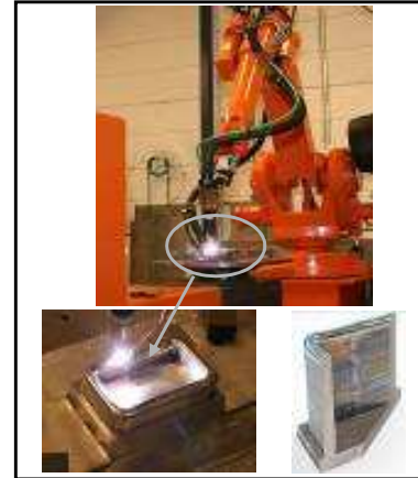
Metal deposition trials for cost effective manufacturing of relevant features for active cooling air cooling on a combustor case
